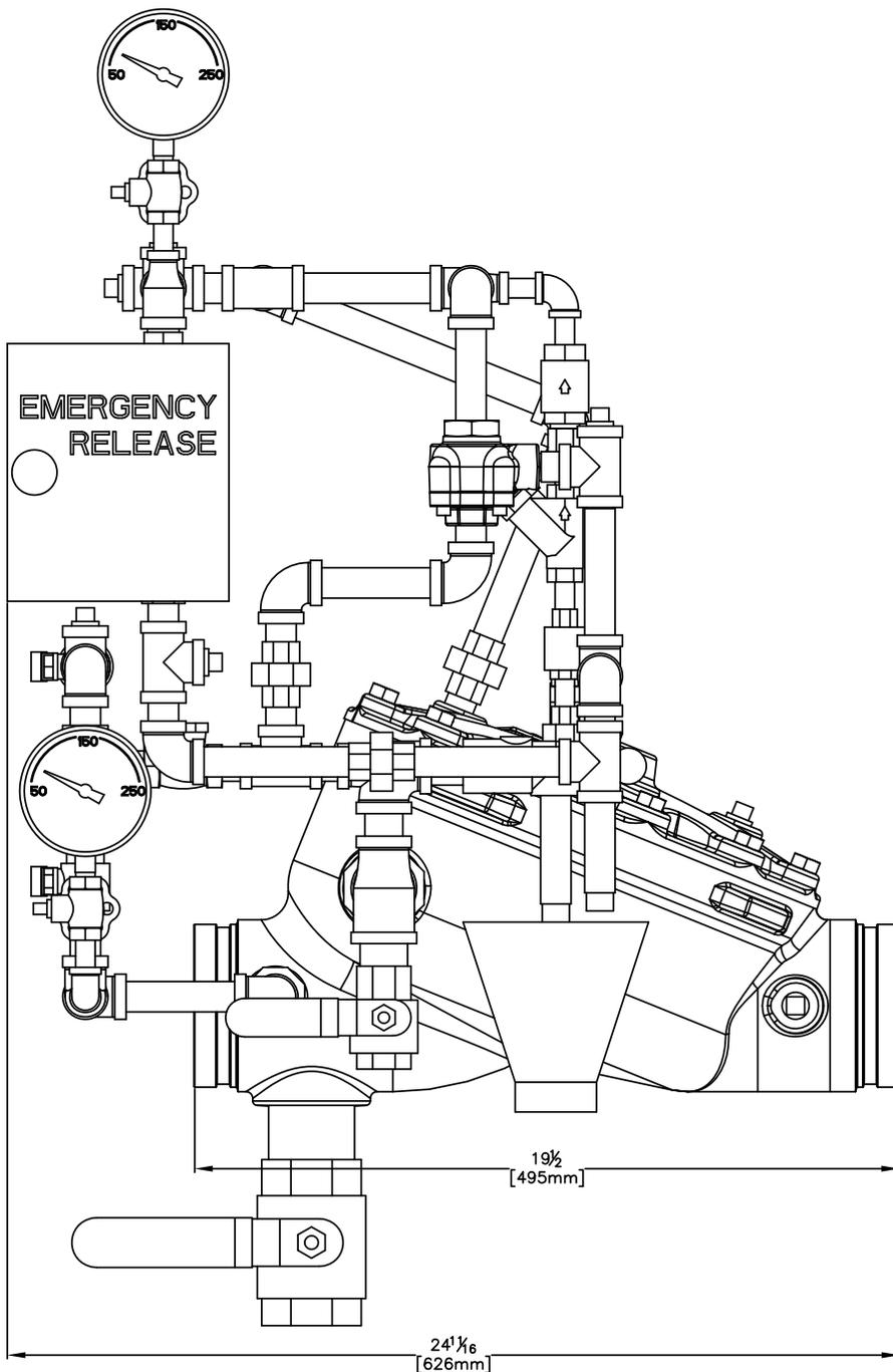
Figure 3a: Installation Dimensions
