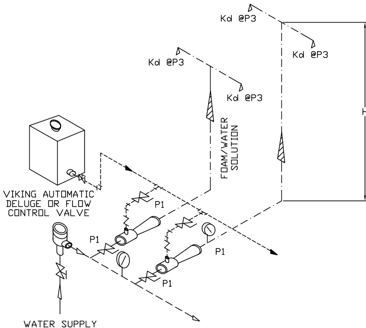
**FIGURE 1 - LOW PRESSURE (50-90 PSI) FIXED EDUCTOR**
