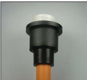
Figure 1: Attach the tool to the end of the CPVC pipe.
