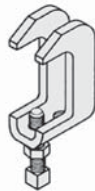
Fig. 66 Steel Reversible "C" Type Beam Clamp with Lock Nut 1 1/4" Opening MSS-SP-69, Type 19 & 23 WW-H-171E, Type 23 Page 28
