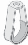
Fig. 2FWON Adjustable Band Hanger w/o Swivel Nut with Felt Lining MSS-SP-69, Type 10 WW-H-171E, Type 10 Page 10
