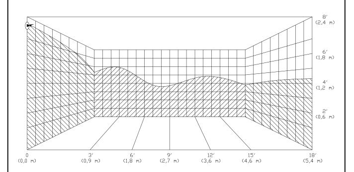
Typical profile of one half of the 16'  $\times$  18' (4,8 m  $\times$  5,4 m) spray pattern produced by a Viking 3/4" (20 mm) Horizontal Extended Coverage Sidewall Sprinkler SIN VK606 installed with the deflector located 4" below the ceiling. Nominal U.S. K-Factor = 8.0 (11,5 metric).
