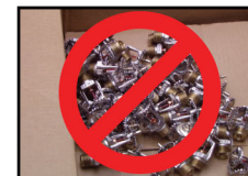
INCORRECT (Stored loose in a box)
