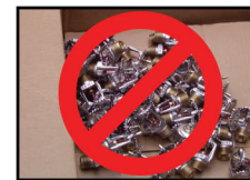
INCORRECT (Stored loose in a box)
