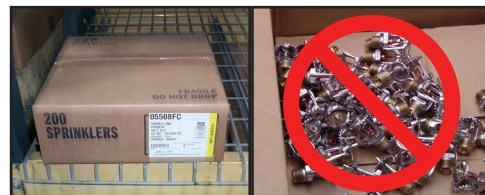
CORRECT (Original container used)
