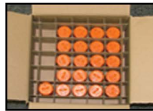
CORRECT (Protective caps in place)
