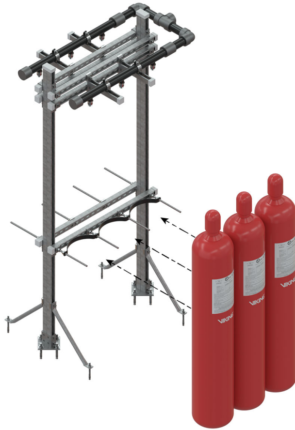
Figure 6.3: Position extinguishing agent cylinders
