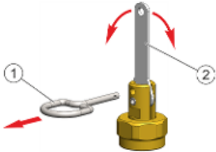
Figure 9.36: Activating the manual release device
