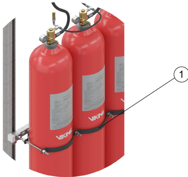
Figure 12.7: Removing the mounting brackets
