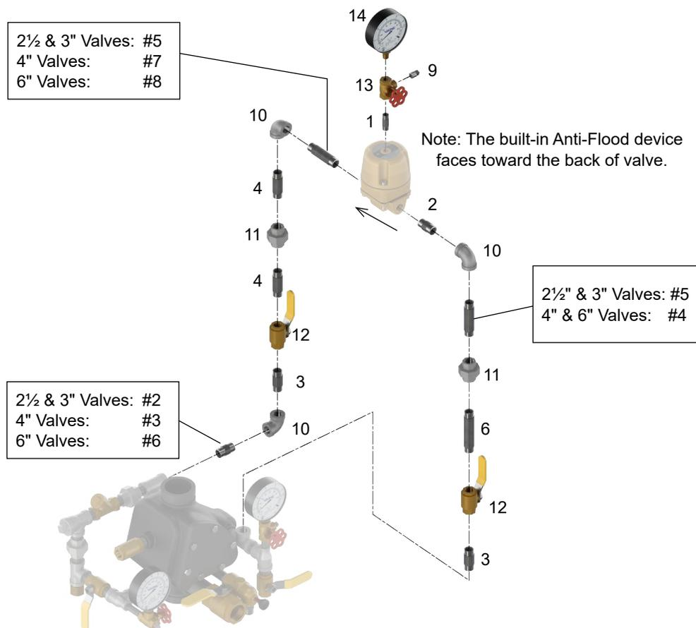
Figure 18: Accelerator (Model D-2) Trim Diagram - 2½" Shown
