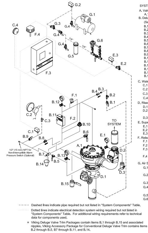
FIGURE 1: ANGLE DELUGE VALVE WITH TANK-MOUNTED COMPRESSOR (6" Valve Shown)
