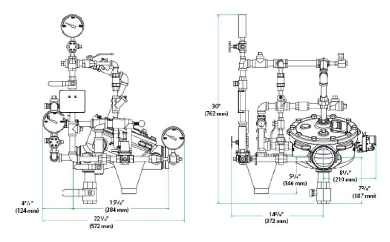
Figure 3 - Installation Dimensions
