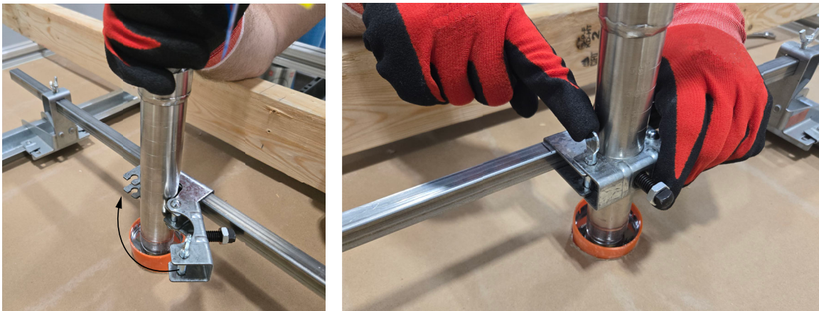
Figure – 4: Close Hinge Door and Locking Shaft
