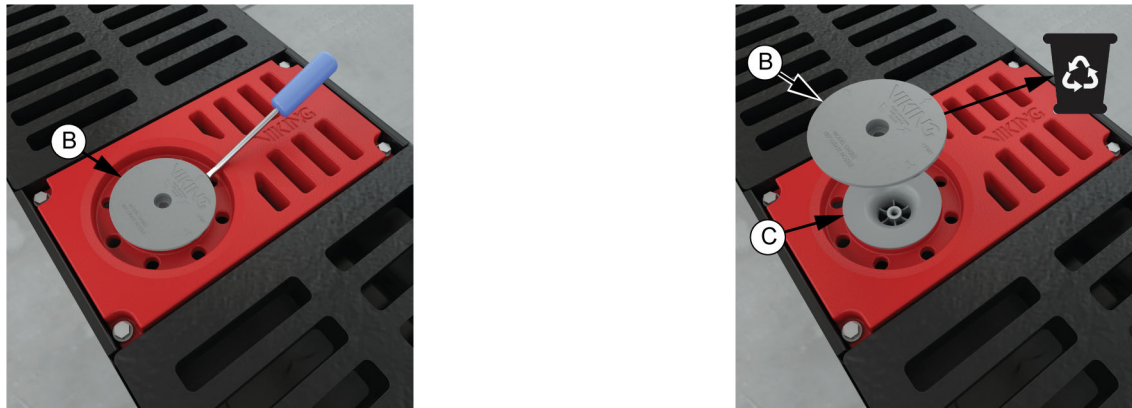
Figure – 4 Removing the Existing Nozzle Deflector
