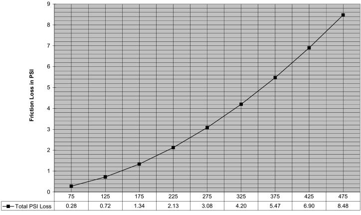
Flow in GPM (C = 120)
