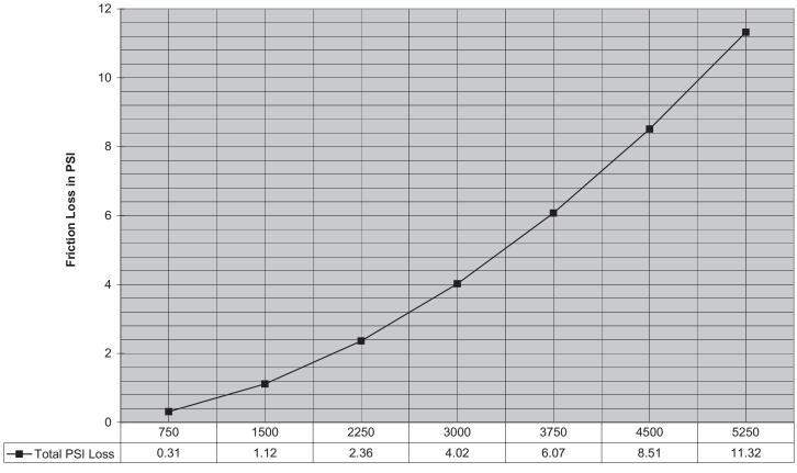
Flow in GPM (C = 120)
