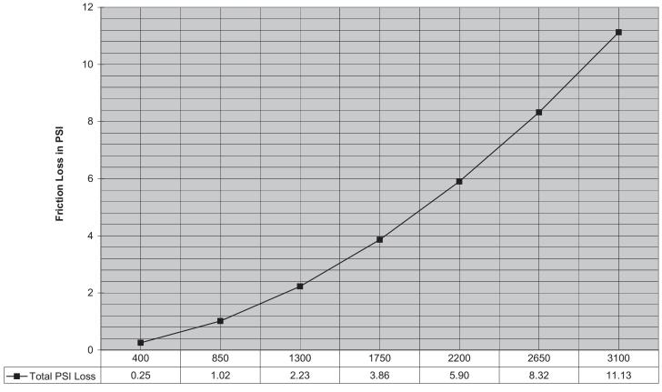
Flow in GPM (C = 120)
