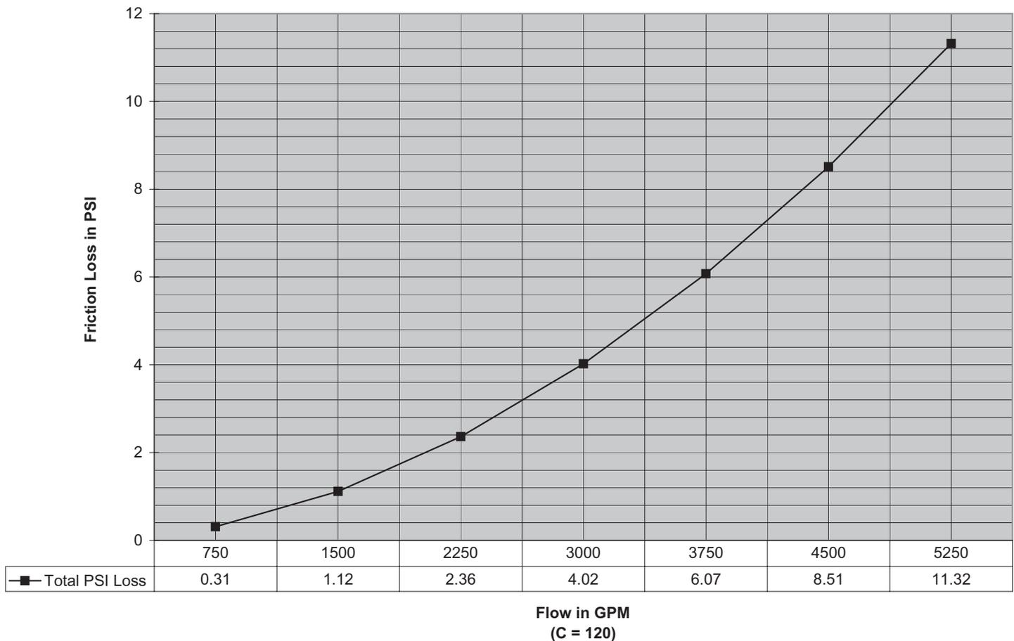
**Friction Loss for the 8" Viking Model J Series Flow Control Valves is equivalent to 57 feet of 8" Schedule 40 (id = 7.981") Pipe (C = 120).**
