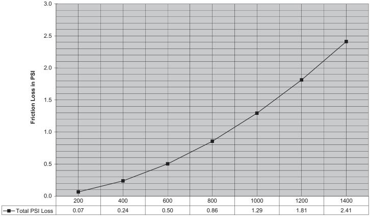
Flow in GPM (C = 120)
