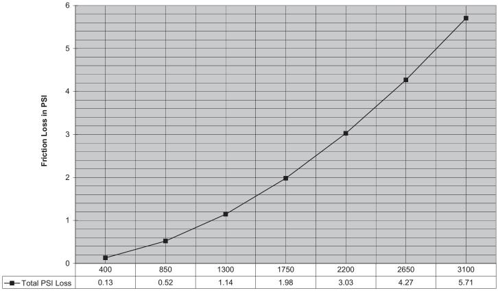
Flow in GPM (C = 120)
