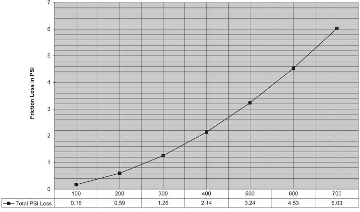
Flow in GPM (C = 120)
