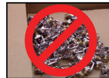
INCORRECT (Stored loose in a box)
