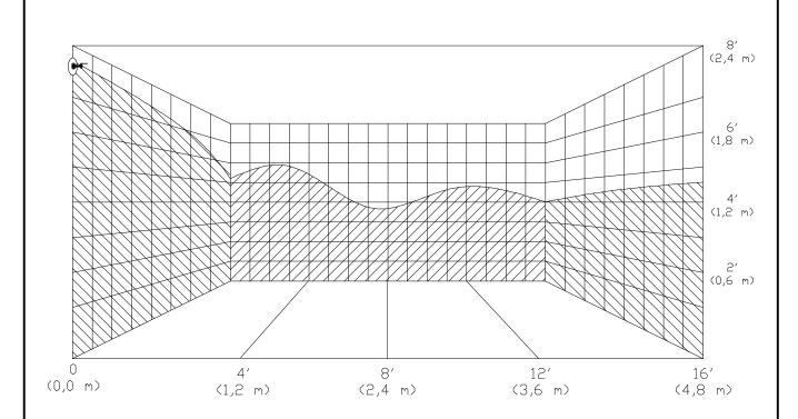
Typical profile of one half of the 16'  $\times$  16' (4,8 m  $\times$  4,8 m) spray pattern produced by a Viking 3/4" (20 mm) Horizontal Extended Coverage Sidewall Sprinkler SIN VK606 installed with the deflector located 4" below the ceiling. Nominal U.S. K-Factor = 8.0 (11,5 metric).
