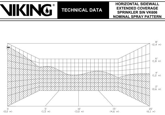
Typical profile of one half of the 16' x 20' (4,8 m x 6,1 m) spray pattern produced by a Viking 3/4" (20 mm) Horizontal Extended Coverage Sidewall Sprinkler SIN VK606 installed with the deflector located 4" below the ceiling. Nominal U.S. K-Factor = 8.0 (11,5 metric).
