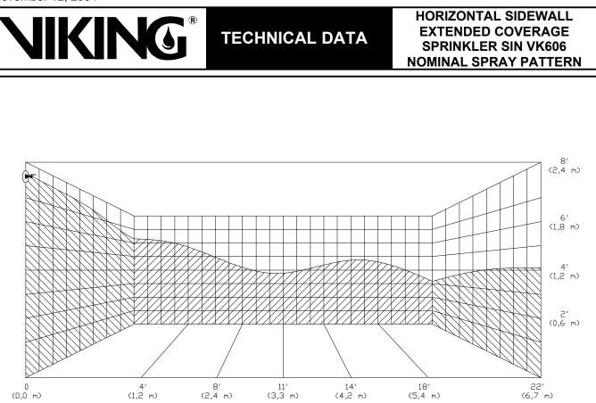
Typical profile of one half of the 16' x 22' (4,8 m x 6,7 m) spray pattern produced by a Viking 3/4" (20 mm) Horizontal Extended Coverage Sidewall Sprinkler SIN VK606 installed with the deflector located 4" below the ceiling. Nominal U.S. K-Factor = 8.0 (11,5 metric).
