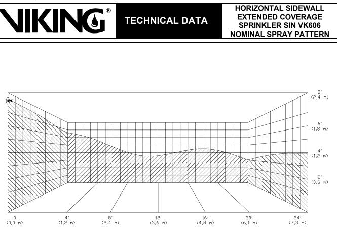
Typical profile of one half of the 16' x 24' (4,8 m x 7,3 m) spray pattern produced by a Viking 3/4" (20 mm) Horizontal Extended Coverage Sidewall Sprinkler SIN VK606 installed with the deflector located 4" below the ceiling. Nominal U.S. K-Factor = 8.0 (11,5 metric).
