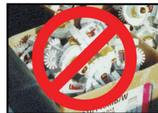
INCORRECT (Protective caps not in place)
