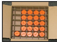
CORRECT (Protective caps in place)
