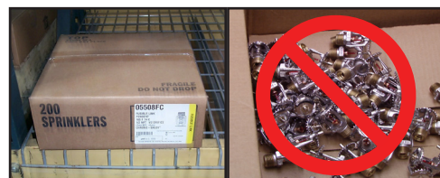
CORRECT (Original container used)
